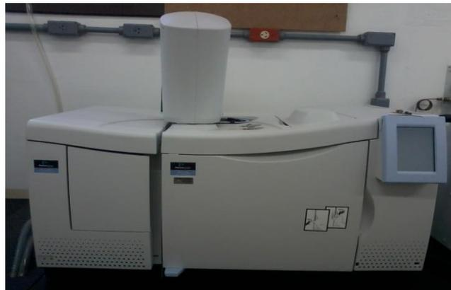
Figura 6: GC – MS Clarus 600 *Perkin Elmer*
