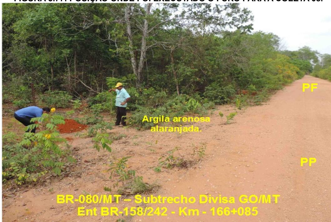
**FIGURA 5.78: CARACTERIZAÇÃO DO PERFIL DE SOLO OBSERVADO NO FURO 08.**
