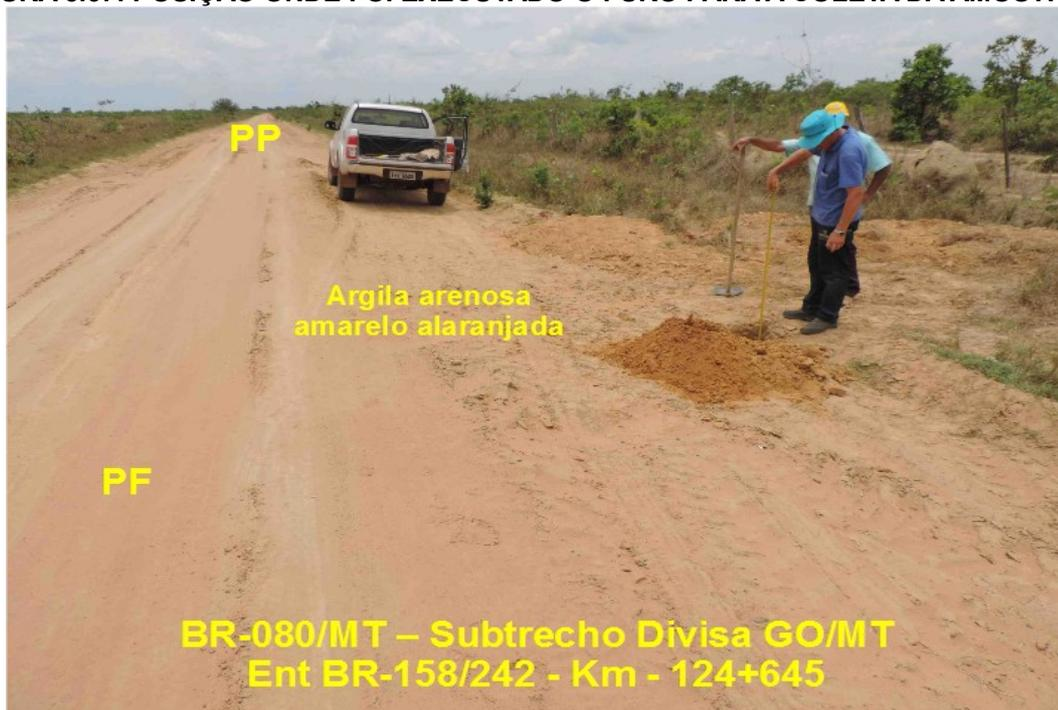
**FIGURA 5.68: CARACTERIZAÇÃO DO PERFIL DE SOLO OBSERVADO NO FURO 03.**
