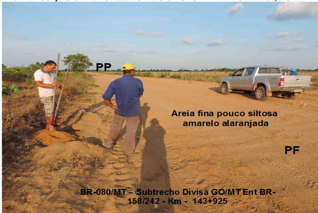
**FIGURA 5.72: CARACTERIZAÇÃO DO PERFIL DE SOLO OBSERVADO NO FURO 05.**
