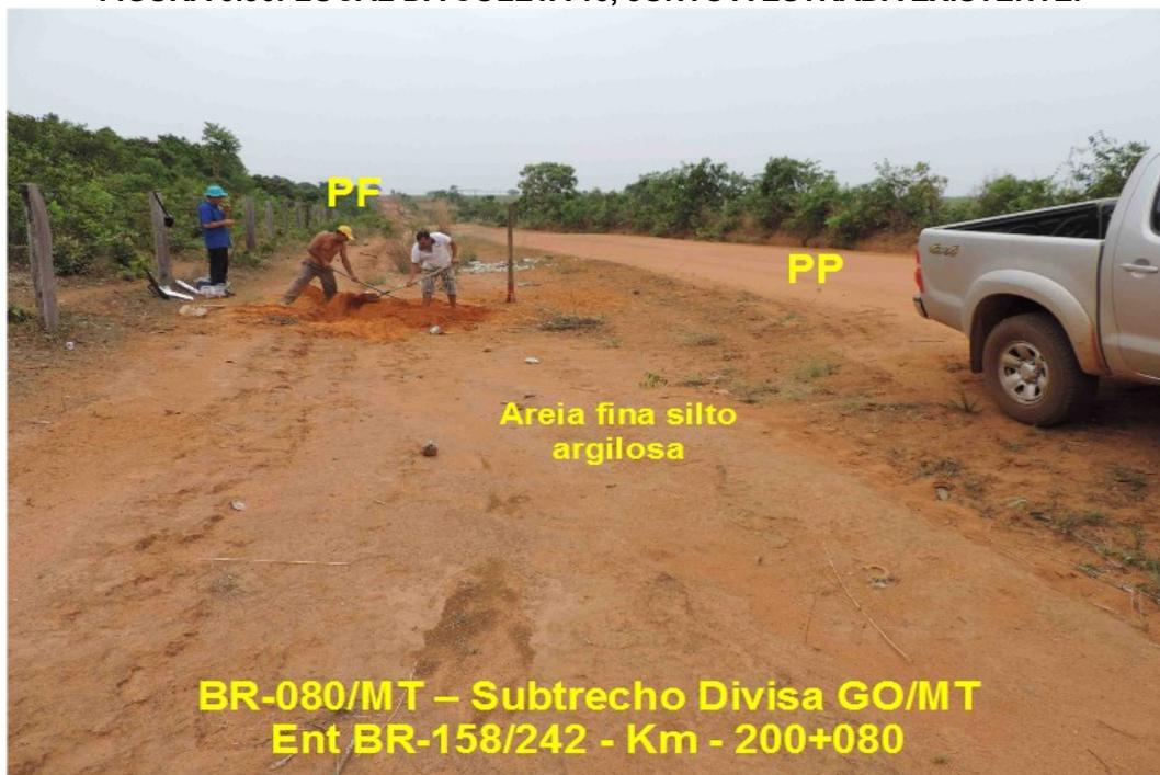
**FIGURA 5.87: CARACTERIZAÇÃO DO PERFIL DE SOLO OBSERVADO NO FURO 13.**
