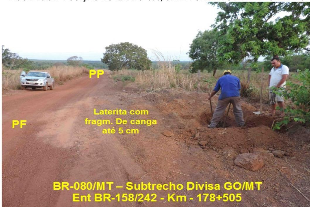
**FIGURA 5.82: CARACTERIZAÇÃO DO PERFIL DE SOLO OBSERVADO NO FURO 10.**
