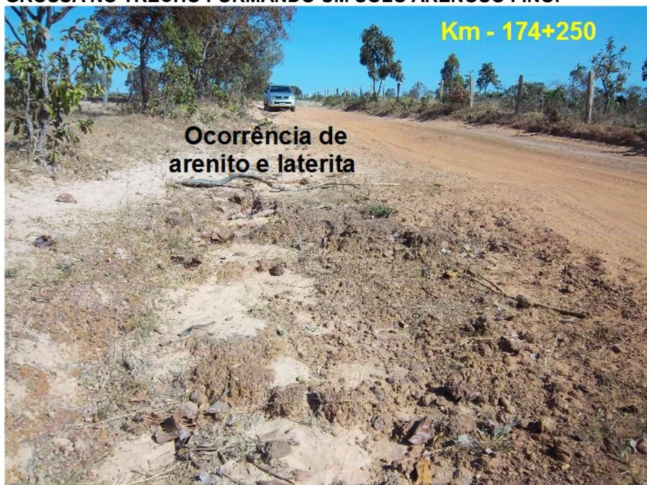
**FIGURA 5.103: SOLO ARENOSO FINO, NO TRECHO DA BR080.**
