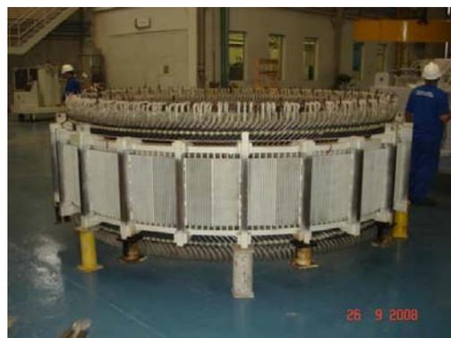
**Figura 3.8:** Estator do Motor (MSA 1)
