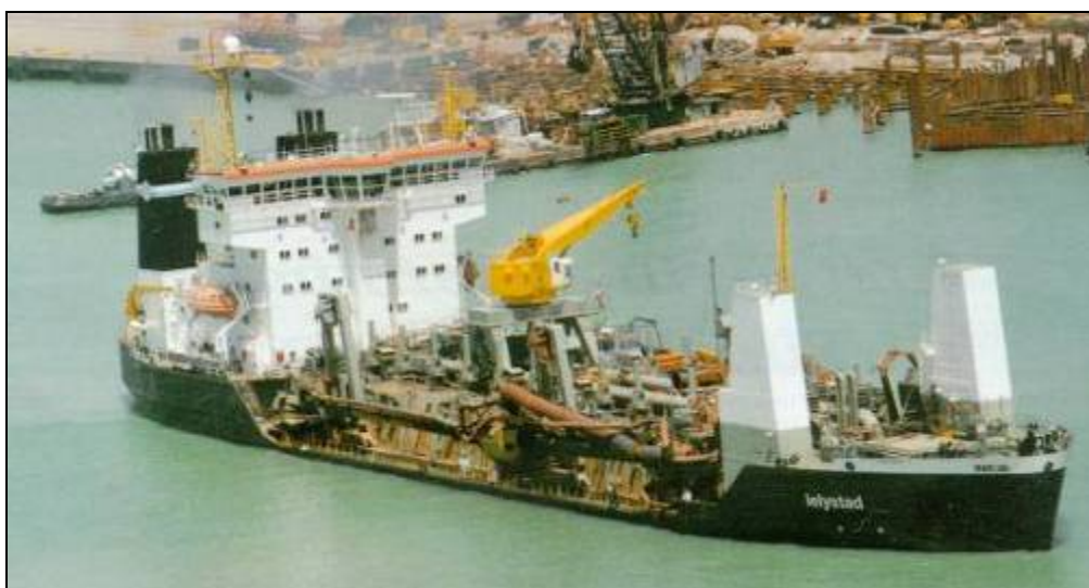
Figura 3.1: Trailer Suction Hopper Dredger (TSHD)
