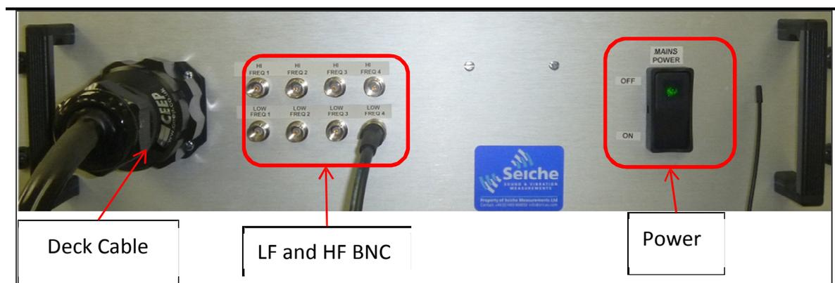
Figura II.9.11-5- Caixa de Buffer (painel frontal)
