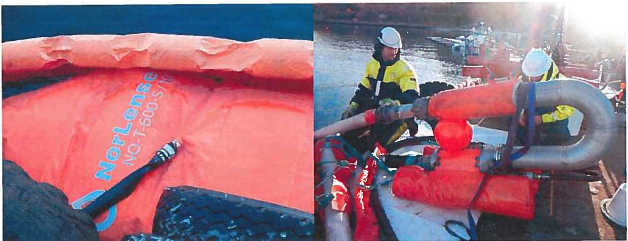
Figure 1 Collection bag NO-T-600-S/NO-T-1000-S (10 m 3 ) (left) and TK 150 pump from Framo (right).
