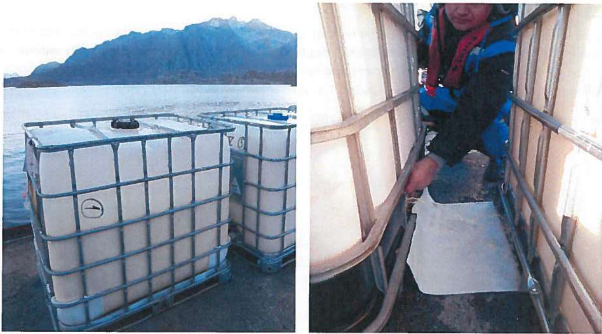
Figure 2 IBC container with soyoil-emulsion (left) and drainage of free water at the bottom of the tank before testing (right).
