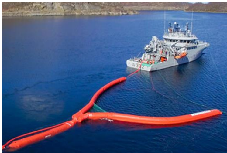
Figure 2: Oil trawl being operated by the Norwegian Coast Guard in an exercise.
