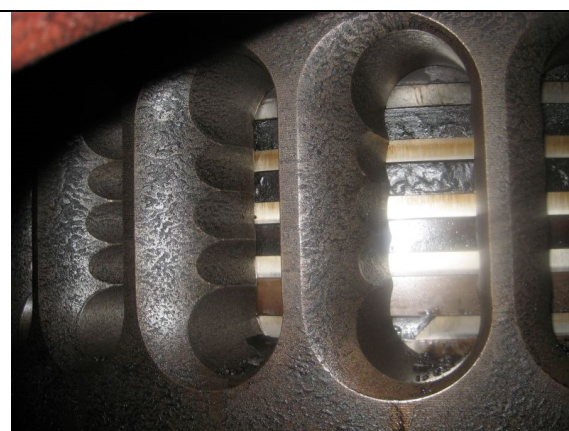
Main engine Cyl 12 broken top ring
