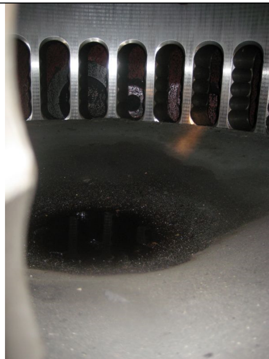
Fuel oil present on top of piston crowns on several cylinder units
