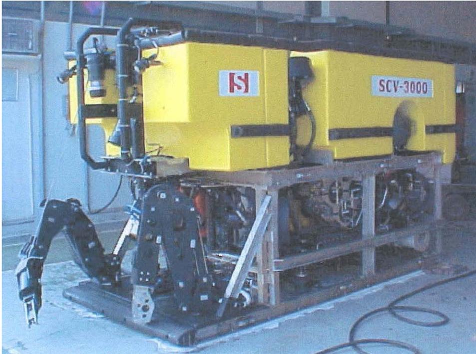
**Figura II.2.4.F-1** - Foto ilustra o ROV (Remote Operated Vehicle).
