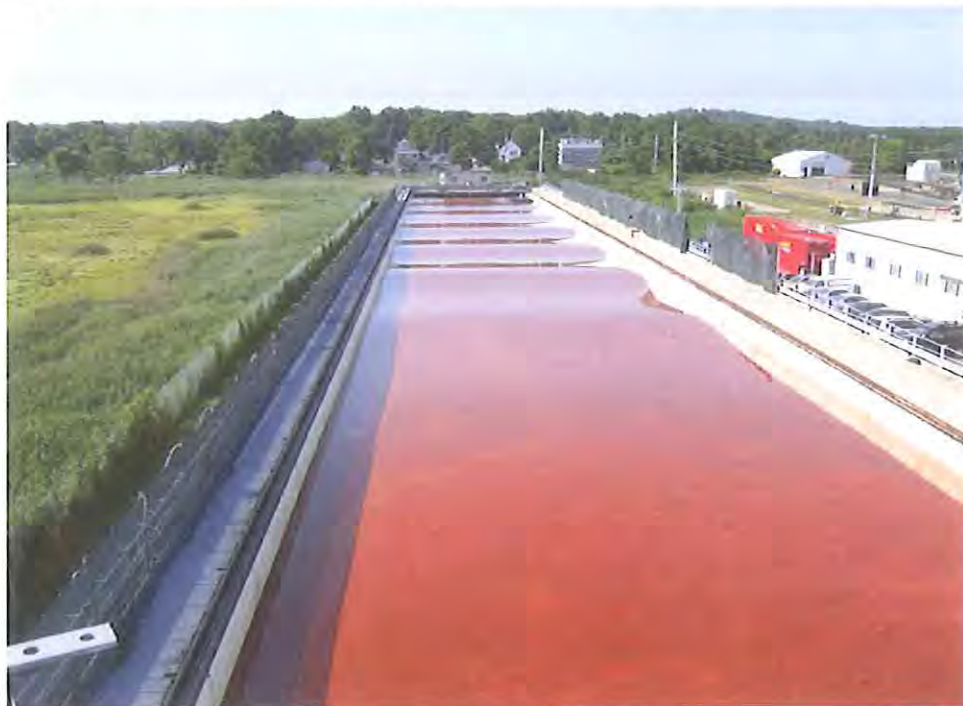
Figure 1 Ohmsett Test Tank with a 25 mm (1 inch) oil layer
