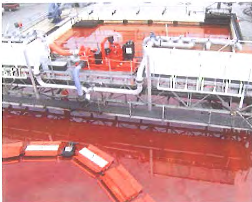
Figure 2 Recovery Tanks on the Auxiliary Bridge
