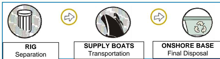
Figure 10 - Solid Wastes Management Scheme.
