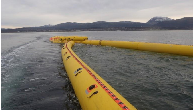
Fig. 2: NOFI Current Buster 6 at ca. 4 knot towing speed
