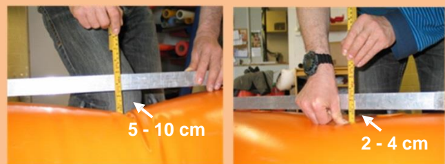
Fig. 22: Testing the overpressure by depressing the air chamber with a knee (left) or a thumb (right).
