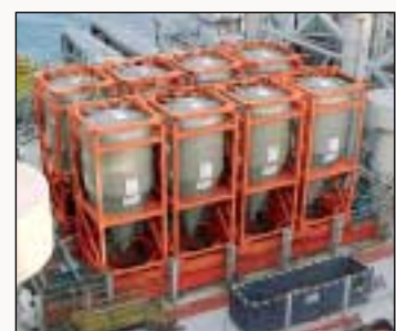
ISO-PUMP units on the rig discharge directly to ISO-PUMP units on the deck of the supply vessel through a flexible hose.
