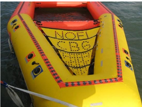
Fig. 13: Splash over protection/wave dampening system in the stern.
