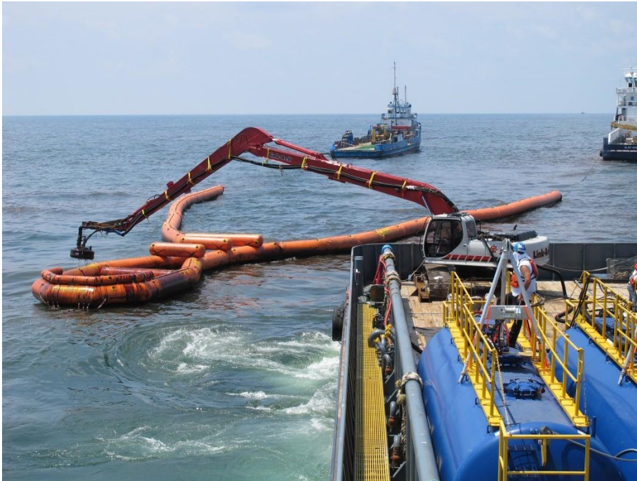
Fig.32: Excavator with pump offloading a NOFI Current Buster 8 during the Macondo spill in 2010.
