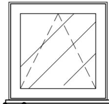
JANELA EM ALUMÍNIO ANODIZADO NATURAL E VIDRO LISO INCOLOR 4mm, TIPO MAXIMAR
