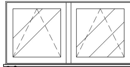
JANELA EM ALUMÍNIO ANODIZADO COM PINTURA ELETROSTÁTICA NA COR BRANCA E VIDRO LISO INCOLOR 4mm, TIPO MAXIMAR
