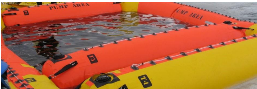
Fig. 20: 3 x 3 m Pump area in the Separator
