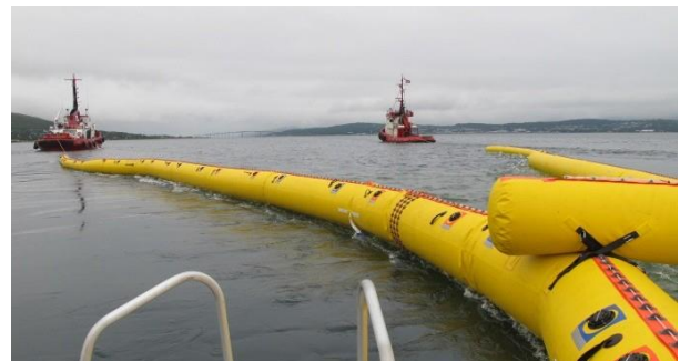
Fig. 26: NOFI Current Buster 6 in a two boat configuration during testing in Tromsø.
