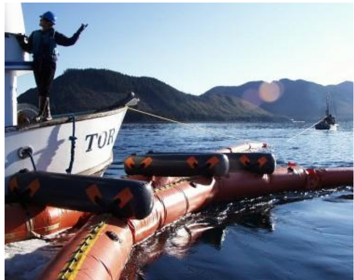
Fig. 31: Mooring line from the bow of the pumping vessel to the connection point between the sweep and the towline. (Image of NOFI Current Buster 4)
