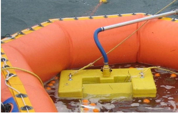
Fig. 28: A skimmer in the separator (Image of NOFI Current Buster 2)
