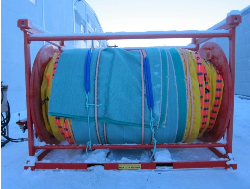
Fig. 21: NOFI Current Buster 6 stored on a 10m 3 boom reel
