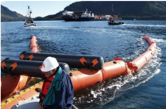
Fig. 33: Turning the system at high towing speed (Image of NOFI Current Buster 4)
