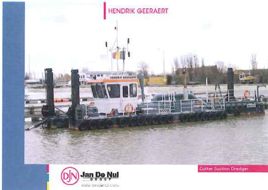
Fig. 2 – Cutter Suction Dredger Hendrik Geeraert
