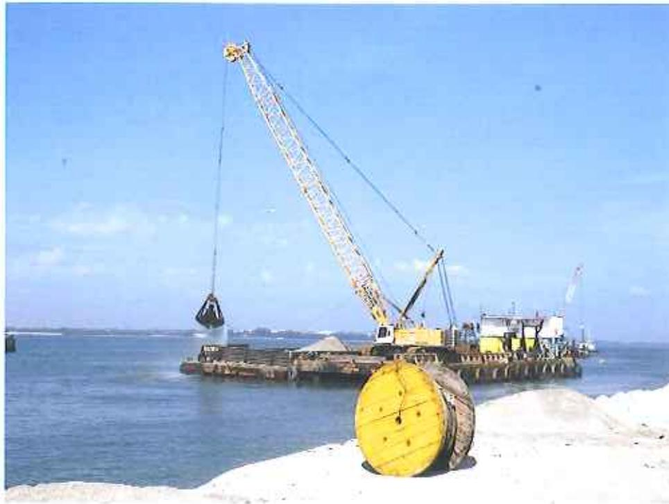
**Fig. 4 - Liebherr HS 895HD on Spud Pontoon DN39**
