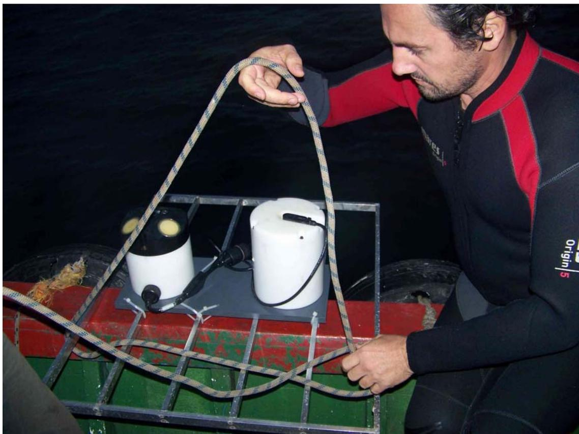
Figura 2: ADP Sontek Argonaut XR 750Mhz
