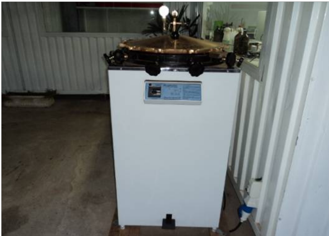
Autoclave vertical, Adamo/PRIS mod. CS 300.
