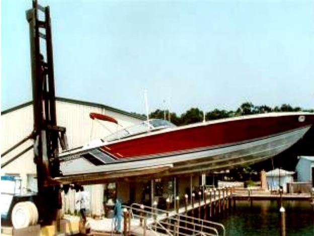
FIGURA 10: E BARCO SENDO RETIRADO DO "DRYSTACK" PELO "FORKLIFT"
