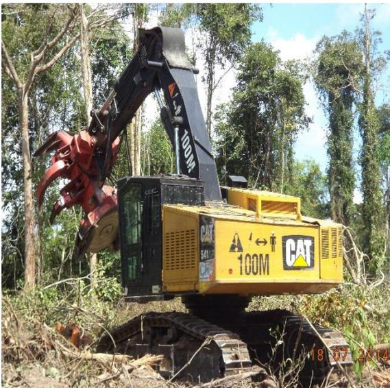
**Figura 12.1.1 - 34 – Corte com feller buncher**
