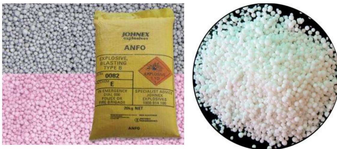
Figura 3.2.2-8 - ANFO (Ammonium Nitrate + Fuel Oil)
