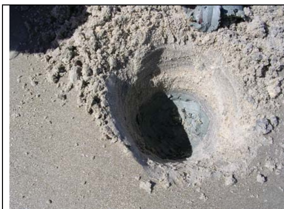
Field Photo 1. Test pit 2 km downdrift of the inlet on the beachface showing a thin veneer of sand covering plastic mud
