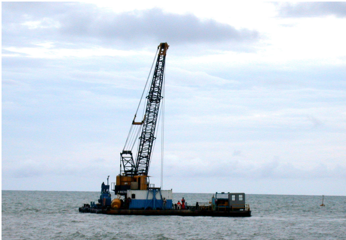
Figura 3.1.3-12 – Flutuante com clamshell
